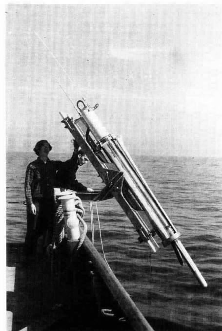
Fig. 5: The author (right) and an undergraduate helper preparing to launch Cox's MSR. A metal can holds down the wing blades and protects the probes. Just below the can is the droppable ballast weight.
