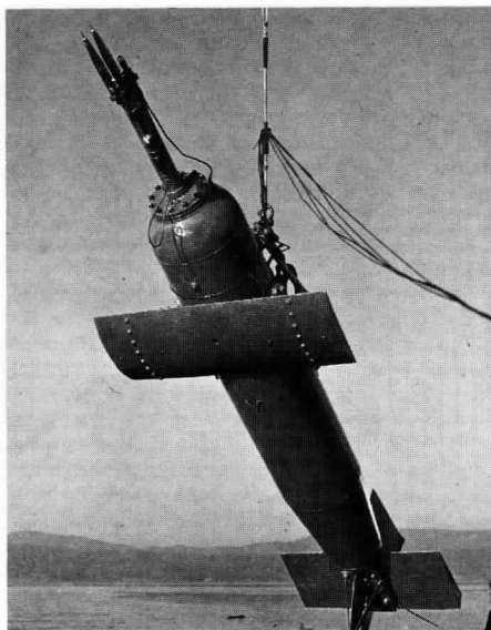
Fig. 1: Paravane Charlie seen from below. The pointed probes at the upper left are a hot film and a cold film. Just behind those two is a thermistor with a protective guard. Below these probes is a small ducted current meter for measuring Charlie's speed through the water. Fig. 2 shows these in detail.
