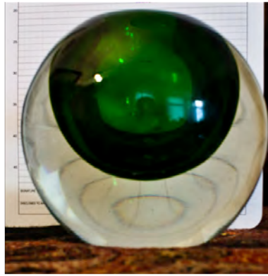
Fig. 2.— Strong lensing by a glass ball at home. The central square of the background paper is distorted. Parallel lines are mapped as semi-arcs, pairs of which make up the ellipses.
