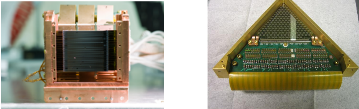
Figure 2: Detector arrays for ACT and SPT. On the left is one of the ACT arrays. It contains 32 by 32 detectors that were fabricated at NASA/GSFC. Cryogenic optics images the sky onto the 32 by 33 mm active area. Each strip of 32 detectors is built onto a silicon card. On the right is an image of a SPT sub array developed at Berkeley. The TES detectors are at the top. Feed horns (not shown) couple the radiation onto the detectors. The circuit board at the bottom contains multiplexing circuitry.
