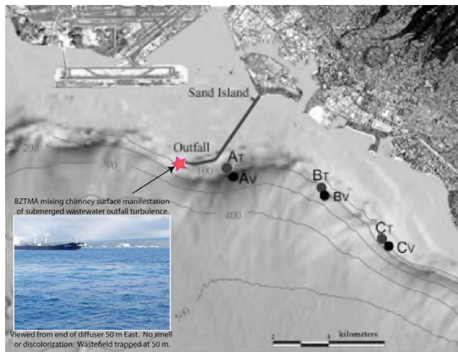
Fig. 1. The schematic for temperature and current velocity measurement stations in Mamala Bay. Insert shows surface manifestations of outfall turbulence trapped at 50 m about 50 m west of the end of the outfall diffuser pipe. Such observable surface smoothing manifestations of the outfall are rare, with little or no discoloration of surface waters and no smell, suggesting their BZTMA (beamed zombie turbulence maser action) mixing chimney origin.
