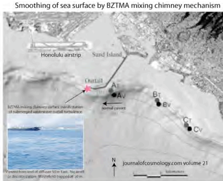
Sand Island outfall in Mamala Bay (Bondur et al. 2015) showing locations of temperature and current velocity measurement stations. Rarely, surface manifestations of the outfall turbulence would appear (red star) about 50 m west of the end of the diffuser pipe, interpreted as a BZTMA (beamed zombie turbulence maser action) mixing chimney. Vertical microstructure profiles showed the turbulent wastewater plume was trapped and fossilized at 50 m below the surface. The observed surface smoothing was accompanied by little discoloration and no smell, proving it was the result of radiated fossil turbulence and zombie turbulence internal waves.
