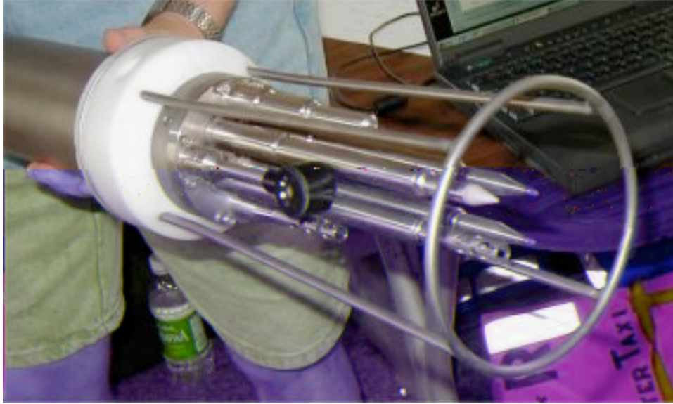
Figure 2: Sensor head of the MSS profiler. The microstructure sensors are mounted on shafts in front of the other sensors. This arrangement guarantees undisturbed measurements of the micro-scale stratification and velocity fluctuations.
