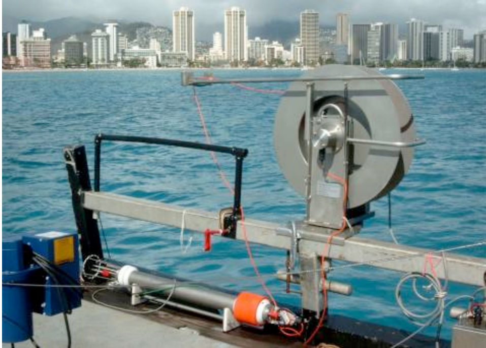
Figure 1: MSS profiler (lying on its side below the railing) and SWM2000 winch in Honolulu Harbour, August 2002.
